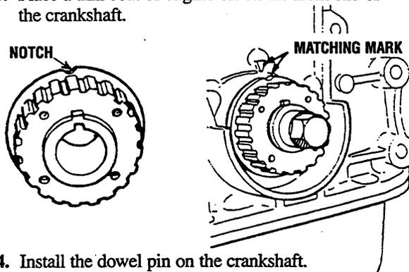
4. Install the dowel pin on the crankshaft.
