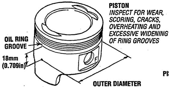
3. Check the piston to cylinder clearance.
