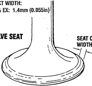
4. Check that the valve seating position is at the center of the valve face.
