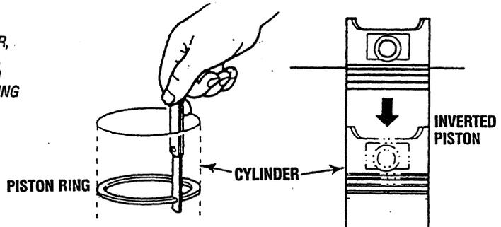
8. Measure the piston ring to ring clearance around the entire circumference using a new piston ring.
