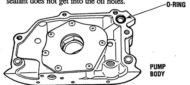
3. Coat the lip of the oil seal with fresh engine oil. When installing the oil seal, be careful not to damage the lip. Tighten the bolts to the specified torque.
