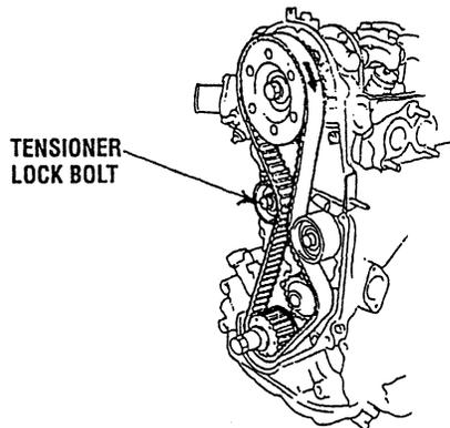
**⚠ CAUTION:** *Water or oil on the timing belt severely reduces the service life of the belt. Keep the timing belt sprocket and tensioner free of oil and grease. These parts should never be cleaned. Replace if seriously contaminated with dirt or oil. If oil is evident on these parts, check the front case, oil pump seals, and camshaft oil seals for a possible leak.*
