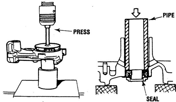
5. Use a pipe to remove the water seal.
