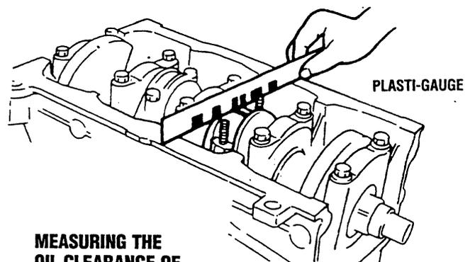
**MEASURING THE OIL CLEARANCE OF THE LARGE END BEARING**
