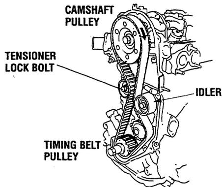
14. Remove the camshaft pulley. Remove the pulley by inserting a T-wrench or similar tool to prevent it from turning.
