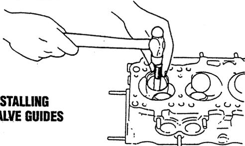
3. Fit the clip onto the valve guide. Use the **valve guide remover and installer** to tap the valve guide in from the side opposite the combustion chamber until the clip just contacts the cylinder head. The height of the valve guide must be **19.1—19.6mm (0.752—0.772in)** from the valve spring seat to the end of the valve guide (dimension A).
