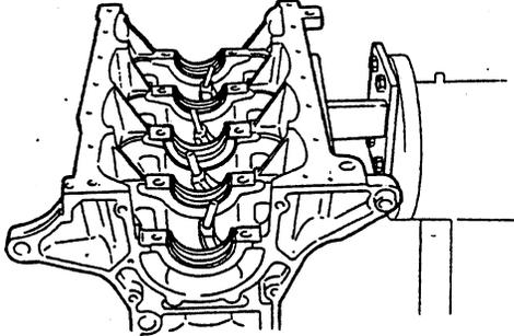
5. Install the main bearing caps in accordance with the numbers and arrows and tighten the bolts to the specified torque.
