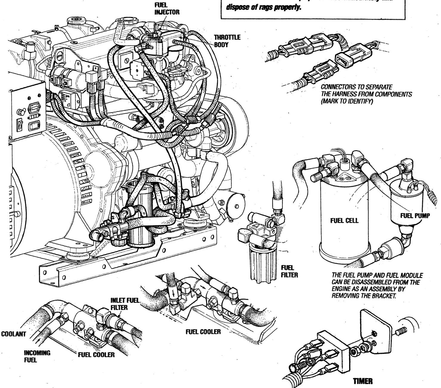
CONNECTORS TO SEPARATE THE HARNESS FROM COMPONENTS (MARK TO IDENTIFY)
