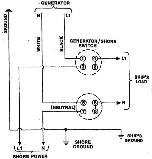
If the installer connects shore power to the vessel's AC circuit, this must be done by means of the Shore Power Transfer Switch. Set the transfer switch shown in the diagrams to the OFF position. This switch prevents simultaneous connection of shore power to generator output.
