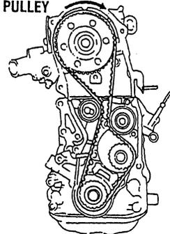
5. Install the timing belt on the crankshaft pulley and the camshaft pulley from the tension side (the right side as viewed from the front of the engine) so that tension is retained.
