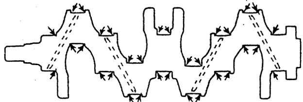
**ALWAYS CHAMFER THE POINTS MARKED WHEN GRINDING THE JOURNALS AND PINS**
