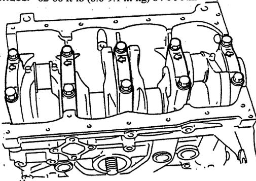
6. Align the connecting rod caps with the match mark.
