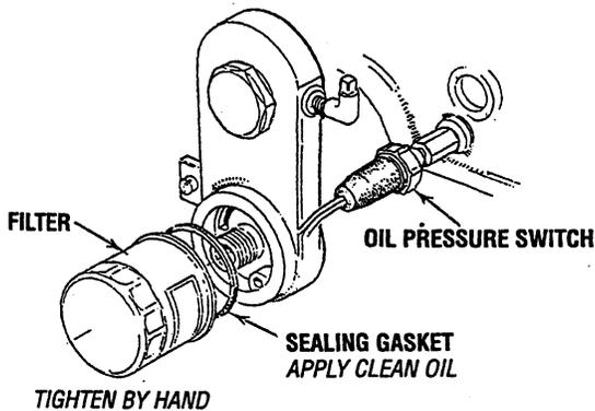
5. Install the oil cooler and oil filter.
