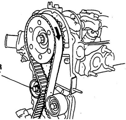
1. Loosen the timing belt tensioner lock bolt and apply spring tension to the belt.
