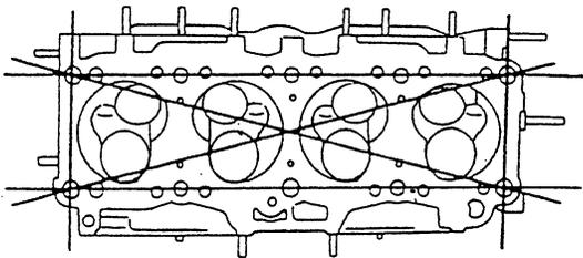
If the cylinder head distortion exceeds specification, grind the cylinder head surface.
