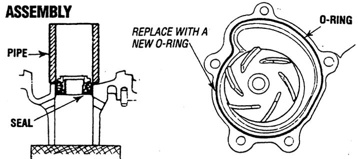
1. Install the water seal by tapping as shown above.
