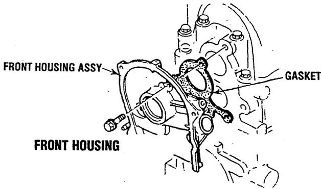
1. Remove the front housing assembly by removing the bolts and nuts.
