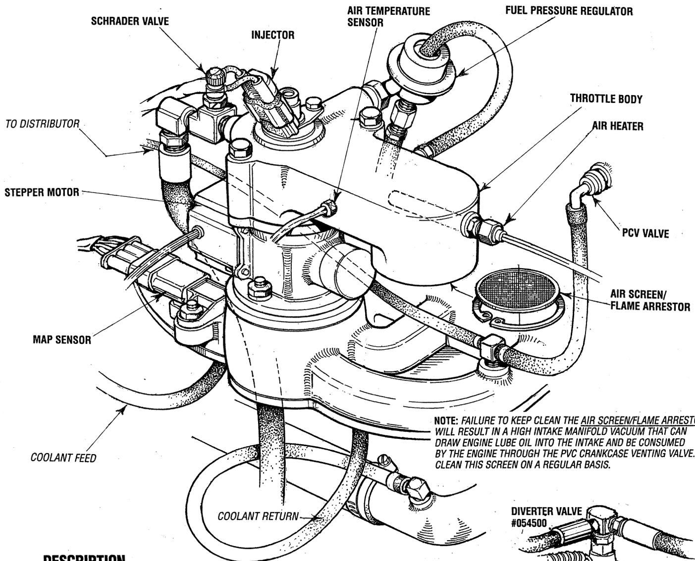
**NOTE:** FAILURE TO KEEP CLEAN THE AIR SCREEN/FLAME ARRESTOR WILL RESULT IN A HIGH INTAKE MANIFOLD VACUUM THAT CAN DRAW ENGINE LUBE OIL INTO THE INTAKE AND BE CONSUMED BY THE ENGINE THROUGH THE PVC CRANKCASE VENTING VALVE. CLEAN THIS SCREEN ON A REGULAR BASIS.
