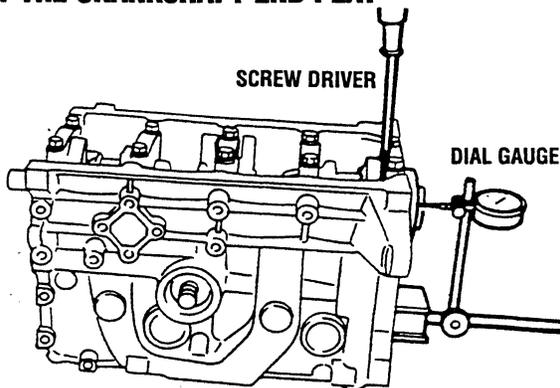
1. Check the end play by moving the crankshaft forward and backward as shown using a magnetic base and dial gauge to measure the amount.
