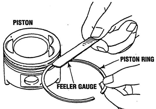
**NOTE:** If replacing piston rings check the piston ring gaps. New rings are packaged with detailed instructions that often supersede the service manual.
