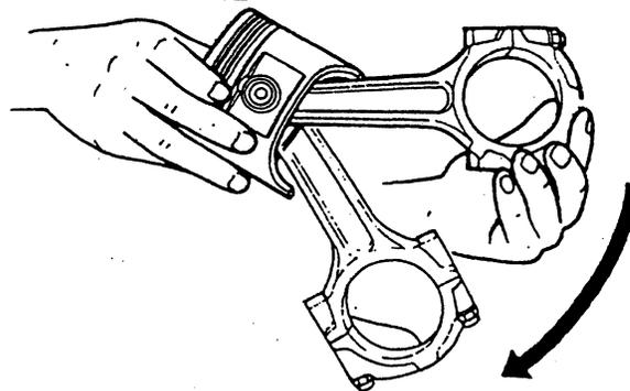
5. After pressing the piston pin in, swing the large end of the connecting rod upward and release it. The connecting rod must swing downward freely.
