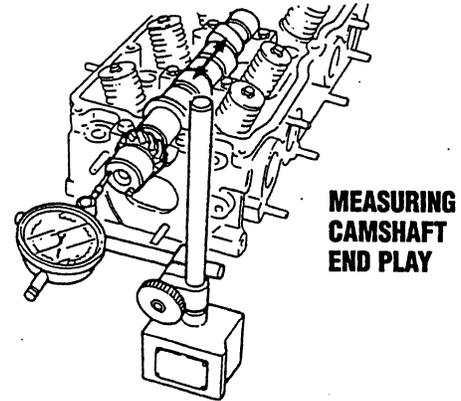
6. Measure the camshaft end play. If the end play exceeds specification, replace the camshaft and/or the cylinder head.
