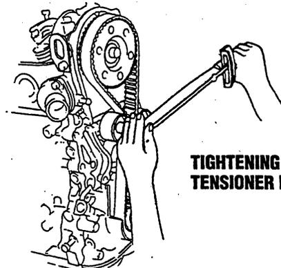
TIGHTENING THE TENSIONER LOCK BOLT
