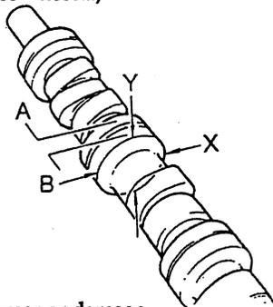
4. Inspect the fuel cam for wear or damage.
