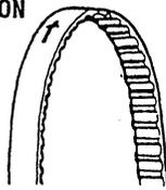
IF RE-USING THE TIMING BELT, INSTALL IT IN THE DIRECTION OF THE APPLIED ARROW - FORWARD ROTATION.
