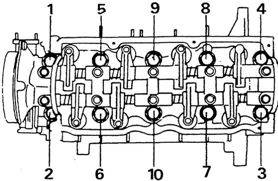
1. Loosen the cylinder head bolts in several increments to remove, following the numerical sequence indicated above.
